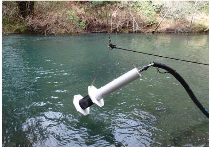
A California Department of Fish and Wildlife-compliant submersible pump fish screen. Photograph courtesy of Sanctuary Forest, Inc.
