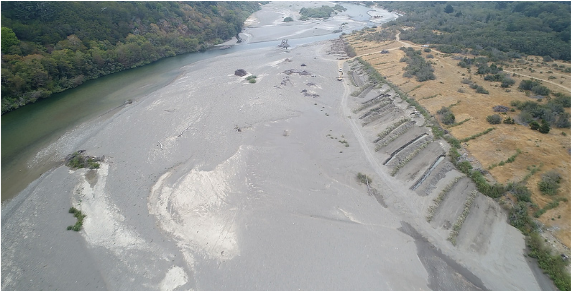
Above: Drone photo of trenched willow installed in 2015 (on bank,) 2016 (upper floodplain terrace,) and 2017 (lower floodplain/gravel bar). Photograph courtesy of Sonny Anderson.
